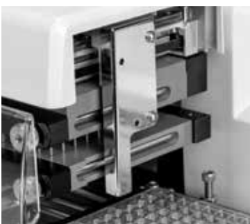
The Agilent BioTek Verify module is built in above the manifold and determines the fluid volumes in each well following dispense and aspirate cycles.
