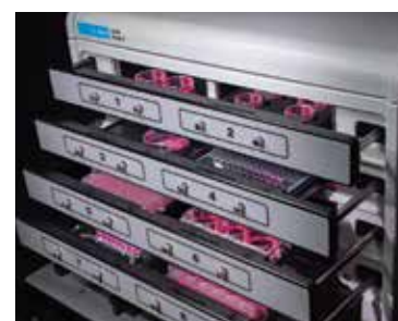
The Agilent BioTek BioSpa 8 automated incubator processes up to eight microplates or other labware at a time.
