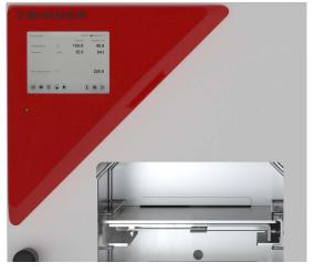
VDL models are equipped with a touchscreen controller allowing digital setting of temperature and pressure.
