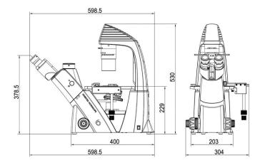
Measurements are in mm, overall dimension may change slightly depending on model
